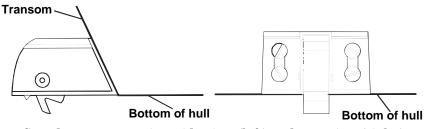
Speed sensor mounting: side view (left) and rear view (right.)
